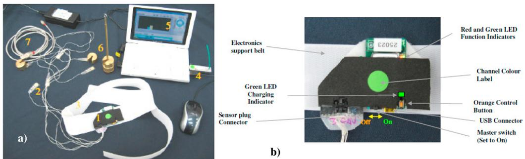
Fig. 1. a) Wearable pressure monitoring system, b) System transmitter features.
