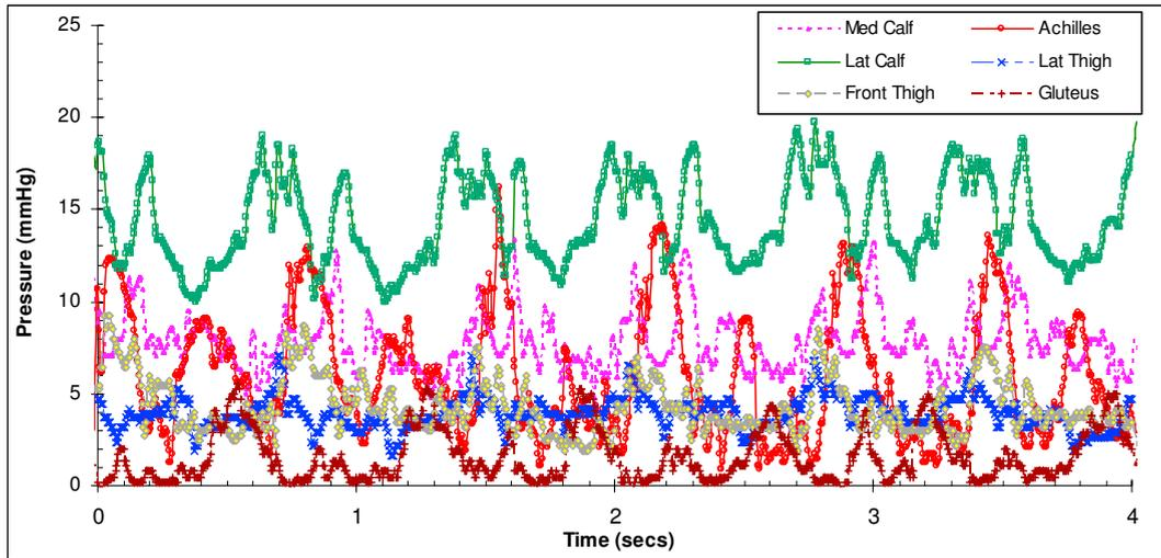
Fig. 5. Variation in garment pressure during running at various positions as measured with the wearable dynamic pressure monitoring device.
