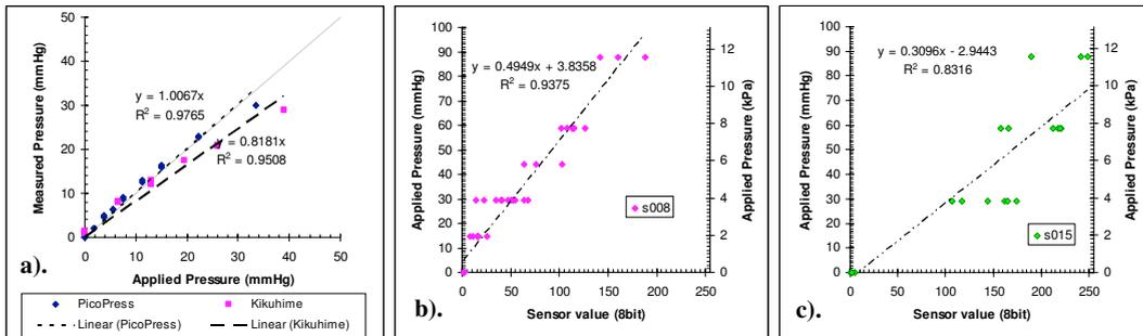
Fig. 4. Sensor calibration and characterization a) Kikuhime™ and PicoPress™, b) Modified Flexiforce sensor with unacceptable precision, and c) Modified Flexiforce sensor with poor linearity and precision.
