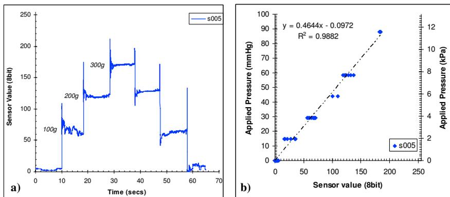
Fig. 3. Sensor characterization, a) Step test result, b) Calibration of sensor value and pressure.
