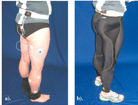
Fig. 2. Wearable dynamic pressure monitoring device on subject, a) No garment, b) Under garment.
